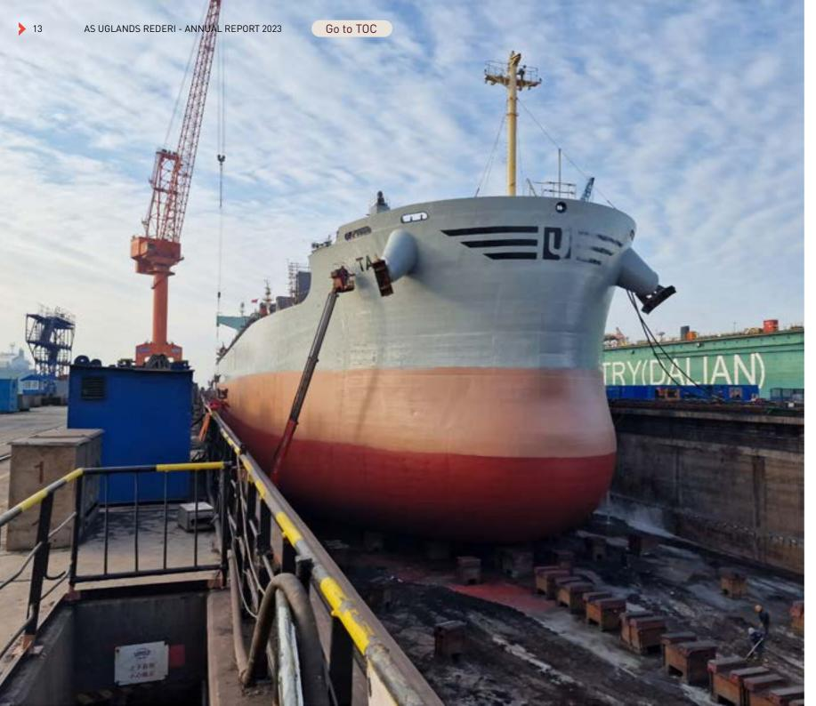
Kristinita receiving new coats of low-friction paint following thorough sand blasting of the hull at Cosco Dalian Shipyard, China.
